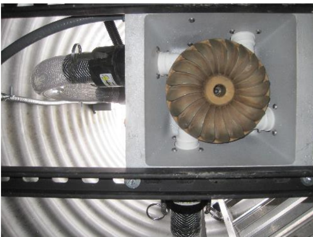
ES&D Stream Engine Turgo runner, 4 nozzles
