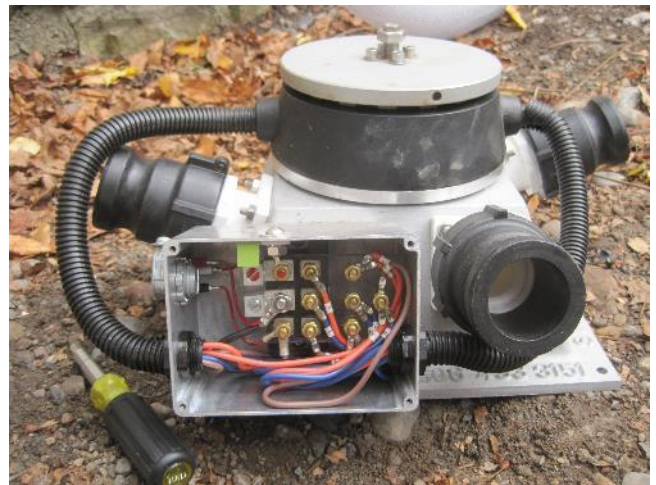
ES&D Stream Engine 1 kW hydro turbine
